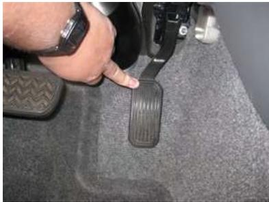
Toyota case was due to potential problems with the gas pedal mechanism that can cause the accelerator to become stuck - regardless of whether the vehicle contains a floor mat. Toyota said in certain rare cases, the gas pedal mechanism wears down, causing the accelerator to become harder to press, slower to return or, in some cases, stuck. The gas pedals was too long and there is a little space between it and the floor mat. In all, there was a poorly designed floor mat
